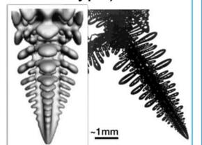
Dendritic growth: simulation [2] and experiment (*mix.msfc.nasa.gov*)
