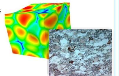
Gradient plasticity: simulation and experiment [3]
