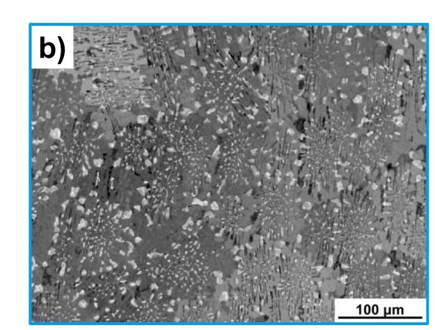
SEM-BSE images of a) longitudinal cross-section and b) transversal cross-section with colonies of ternary eutectics directionally solidified at 60 mm/h (Hasemann, 2014)
